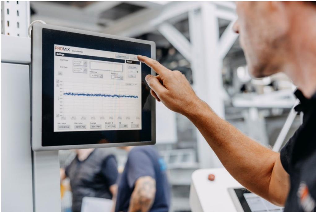
Caption The inline viscometer "Visco-P" measures the actual viscosity of the melt under process conditions in real time
