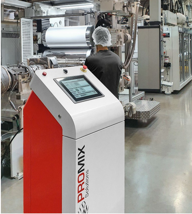
Caption Promix Microcell Technology on an extrusion line for packaging films
